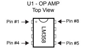
Note: Ensure the IC chip U1 (LM358) is wired correctly. The location of Pin #1 is shown above.
