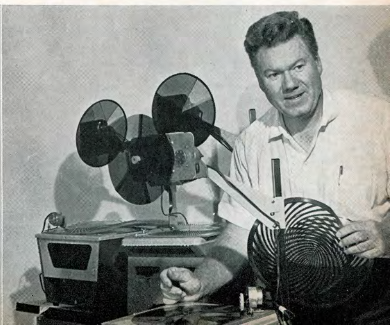
(LEFT) FIGURE 8—Miniature strobe unit of the type used in filming the nightclub sequence. Designed to be hand-held, this strobe delivers 15 to 20 times as much light as similar small units used for light shows and “happenings.” (RIGHT) FIGURE 9—The author, BOB BECK, with a cluster of three of the overhead projectors, demonstrating the manner in which they were actually used during filming of “THE TRIP” to throw “psychedelic” patterns onto bodies of actors and walls of the set.
